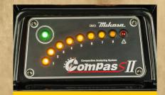
Mikasa 'Compass' compaction meter is a measuring and display system for continuous compaction control - located in clear view of the operator.
