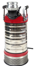
P455D Max flow 1900 L/min Total head 23m Three phase 5.5kW
