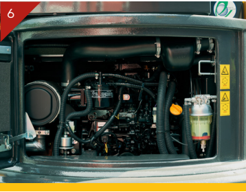
Large rear access for easy engine maintenance
