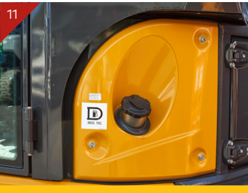
Fuel refill located in a convenient position
