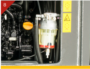
Water separator with indicator
