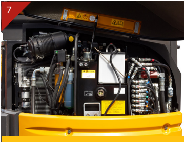
Large side cover for easy service access
