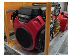
Engine: Honda IGX800 Electric start Pressure 3600psi Max flow 33 L/min
